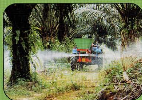
Emdek Mini Turbo Spin (300 kg capacity) mounted on mini-tractor for use on terraces and areas inaccessible to the big tractors. The spreader can be adjusted to apply fertilizers either to the left, right, both sides (as shown) or to the rear of the spreader (Photo taken elsewhere)
