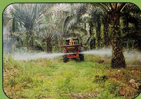
Emdek Turbo Spin (600-800 kg capacity) spreading granular ammonium nitrate covering 4 rows of oil palms in one pass.
