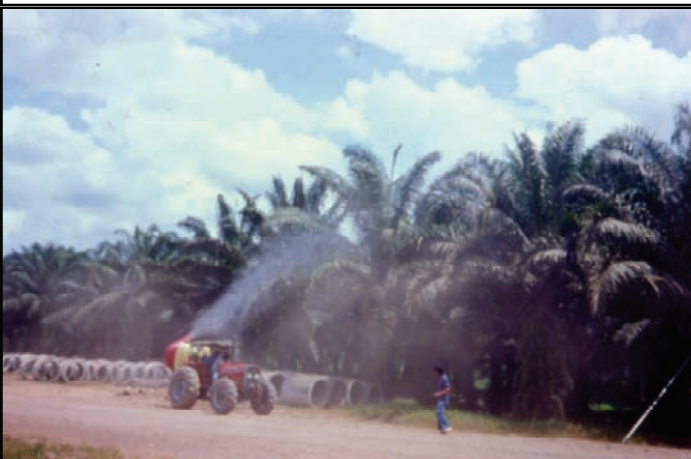
Figure 7. Tractor drawn and driven mistblower for applying insecticide on tall palms.
