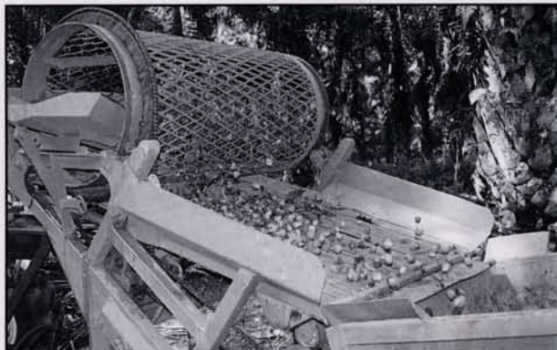
Pamol's prototype trash removal device powered by mini-tractor
