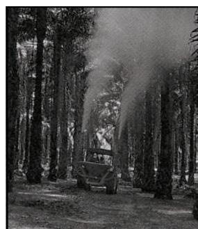
Emdek turbo-spin fertilizer spreader fitted with funnels for sulphur dusting to a height of about 50 feet
