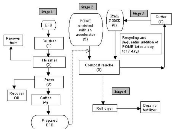
**Figure 2 : Turning POME and EFB into organic fertilizer without producing any waste and discharge**
